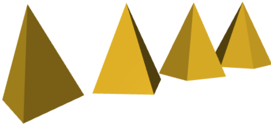
Fig. 32: Pyramids created using the CONE command with r = 5 , h = 10 and m = 3, 4, 5, 6 .
